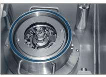
Top view on cutting plate system
