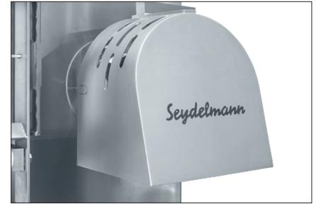
Outlet protection device
